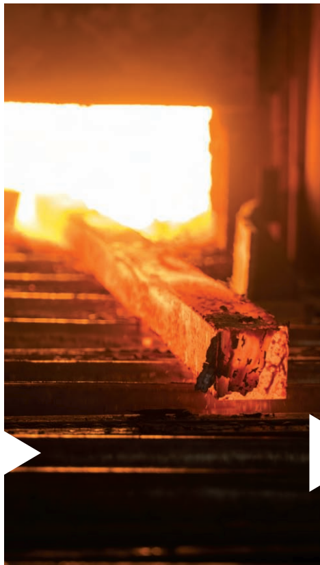
Steel Billet heated in Computerized Controlled Furnace at 1200-1250°C
